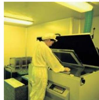
**Angle of the light** - Ideally the light should enter the stencil at an angle of 90° to the positive as this will give no undercutting of the image. Be aware though that the closer the lamp is to the image, the more acute the angle will become at the edges of the image. Ultimately, the size of the screen and the quality of the print you require will determine the optimum distance you should use.
